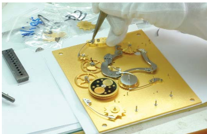
Assembly of the front panel with moon phase indicator.
