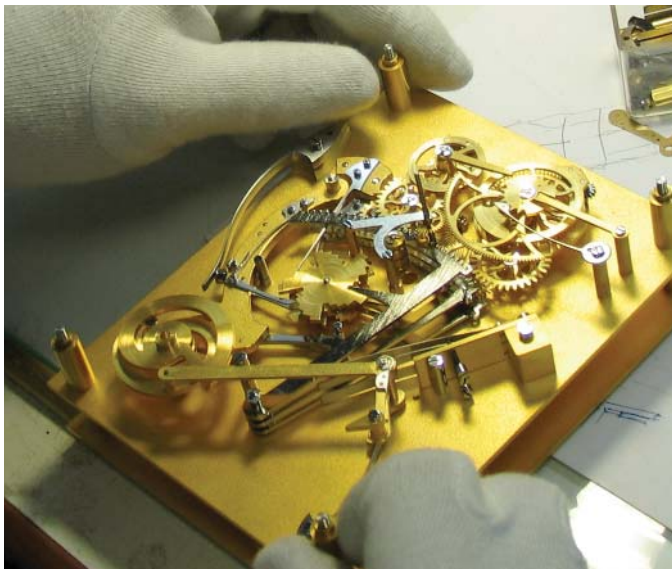
Fully assembled front mechanism with orthodox holidays indicator and perpetual calendars.
